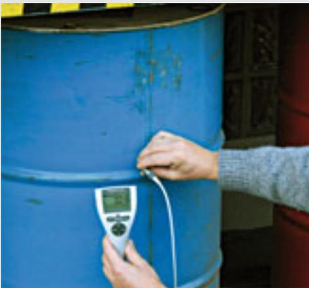
**SIDSP® N and FN sensors compensate for substrate conductivity**
